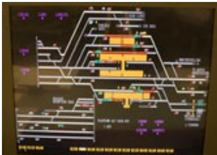
York station is very busy at 1038. To maximise clarity of the station, the route south of Holgate Junction is shown separately in the bottom left-hand corner. The avoiding lines (Slow Lines) don't pass quite so closely to the station and the Scarborough line and ECML are not really parallel.
