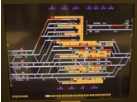
This was Leeds station at 1035 (see text). For terminating services the arriving and departure codes are shown. For example 1A22, 1240 to King's Cross is at platform 6; this had arrived as 1D23, 0935 from King's Cross. The complexity of the west end greatly contrasts with that to the east. It is interesting to see what routes are available from various signals.
