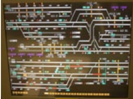
This 'overview' indicates how the ECML south of York is represented on the York South Workstation. In the top left corner, 4R15 from Drax to Immingham has left York's control area near Heck and is now under the supervision of Doncaster PSB. The middle of the screen shows the ECML between Temple Hirst and Hambleton Junctions'. At first it is difficult to reconcile the screen view with the layout on the ground.
